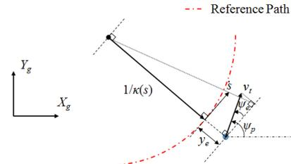
Figure 4. Particle motion description for the vehicle
