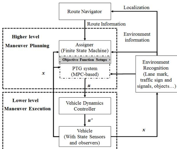
Figure 1. Hierarchical control framework
