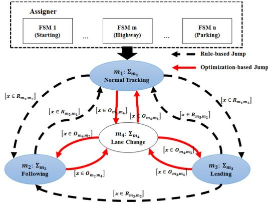
Figure 2. Maneuver automaton in the assigner. Rule-based jump sets are denoted by  $R$  and Optimization-based ones by  $O$ .
