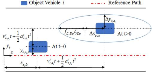
Figure 5. Object motion definition in road reference frame
