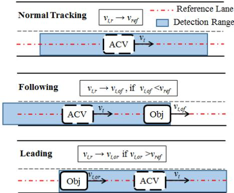
Figure 3. Target speed assignment.
