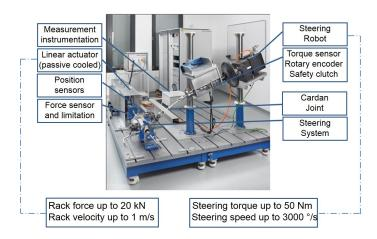
FIGURE 3. DESCRIPTION OF STEERING TEST-RIG
