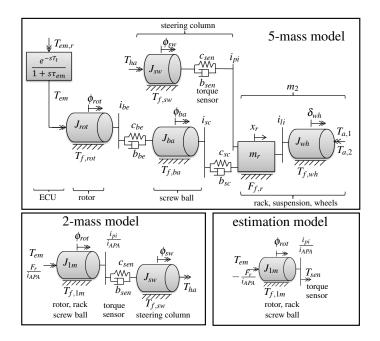
**FIGURE 2**. REDUCTION OF THE LUMPED 5-MASS STEERING SYSTEM MODEL FOR RACK FORCE ESTIMATION
