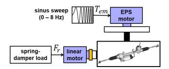
**FIGURE 6**. DESCRIPTION OF TEST PROCEDURE USING STEERING TEST-RIG
