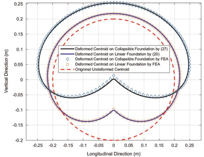
Fig. 3. Comparison of deformed centroid: collapsible foundation vs. linear foundation.
