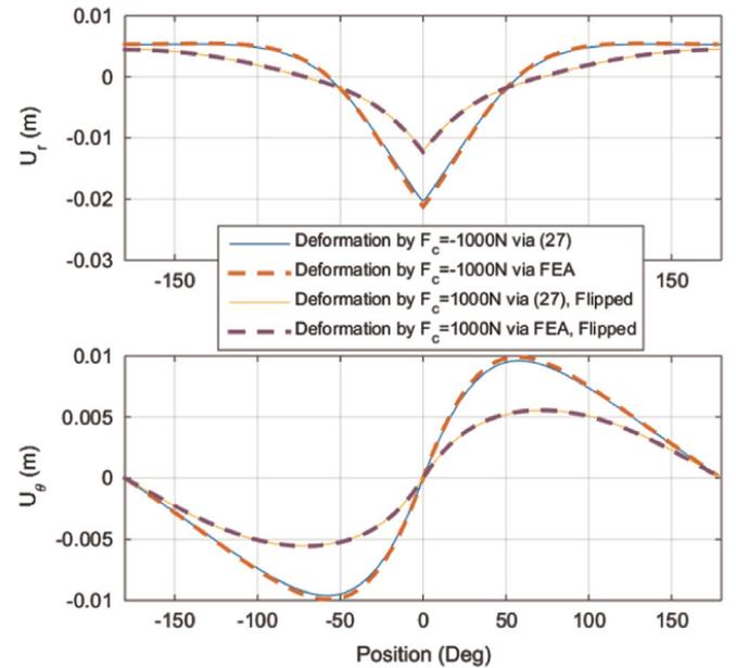
Fig. 4. Comparison of deformed centroid: response by positive and negative force.
