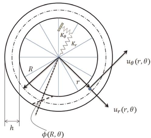
Fig. 1. Thick ring on a two-parameter elastic foundation.
