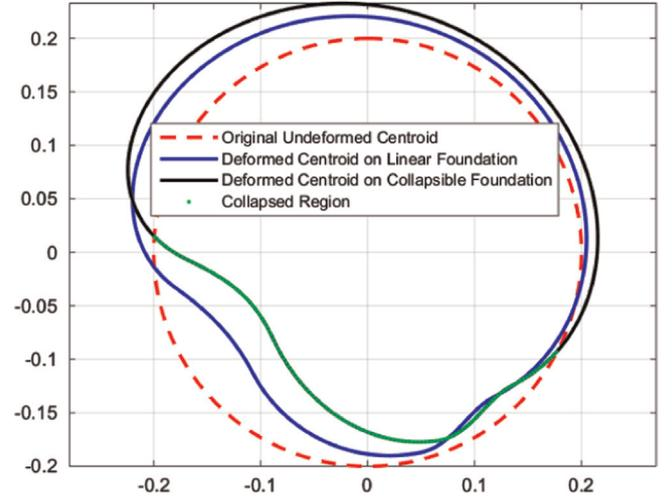
Fig. 6. Deformation of ring centroid due to the distributed force given in Fig. 5.
