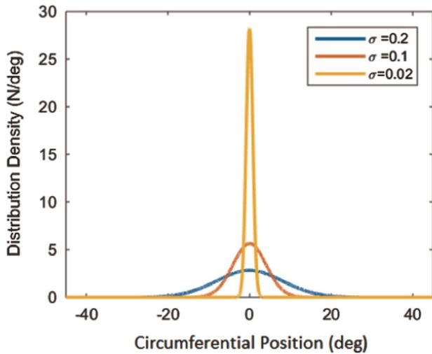
Fig. 2. Effect of  $\sigma$  to the distribution density of a unit force.
