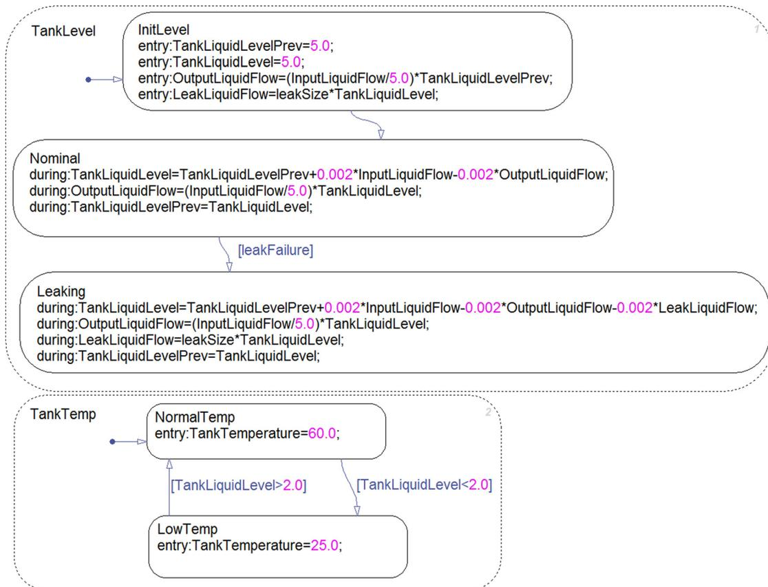
**Fig. 5 Behavioral model of the white liquor tank component**
