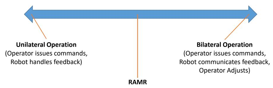
Operator issues commands and adjusts to predicted feedback Robot executes operator intent and handles actual feedback
