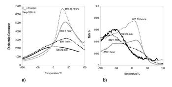
FIG. 3. 650 nm PST on sapphire substrates annealed at 700 °C for 20 min (S=0) and 850 °C for 1 min (S=0), 1 h (S=0.55), and 35 h (S=0.91): (a) dielectric constant and (b) loss tangent at measurement frequency 10 kHz and  $E_{AC}$ =1 kV/cm.
