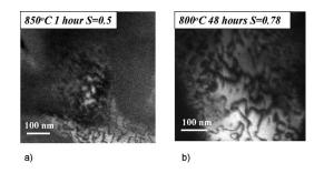
FIG. 2. TEM dark field images (1/2, 1/2, 1/2) of PST on sapphire substrates: (a) films annealed at 850 °C for 1 h (*S*=0.5) and (b) 800 °C for 48 h (*S*=0.78). The diffracted beam from the superlattice was used to image the ordered regions (ordered=white and disordered=black).
