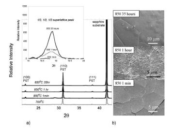
FIG. 1. PST on sapphire substrates (a): X ray of films annealed at 700 and 850 °C for 1 min (S=0), 850 °C for 1 h (S=0.55), and 850 °C for 35 h (S=0.78); (b) SEM determined microstructure films annealed at 850 °C for 1 min, and 1 and 35 h.
