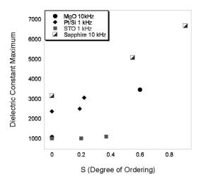
FIG. 4. Dielectric constant maximum vs degree of *B* site ordering for films deposited on (111) Pt/Si (500 nm thick PST), (0001) sapphire (650 nm PST), (111) STO (600 nm PST), and (100) MgO (550 nm PST) substrates.
