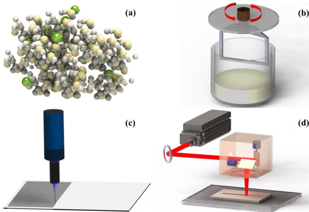
**Fig. 1.** Schematic description of rapid laser reactive sintering (RLRS) process. (a) Mix precursor solids, (b) prepare precursor paste, (c) deposit precursor layer, and (d) perform RLRS.
