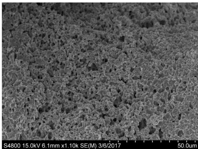
Fig. 7. High magnification porous bottom region of thick BCZYYb layer by RLRS.
