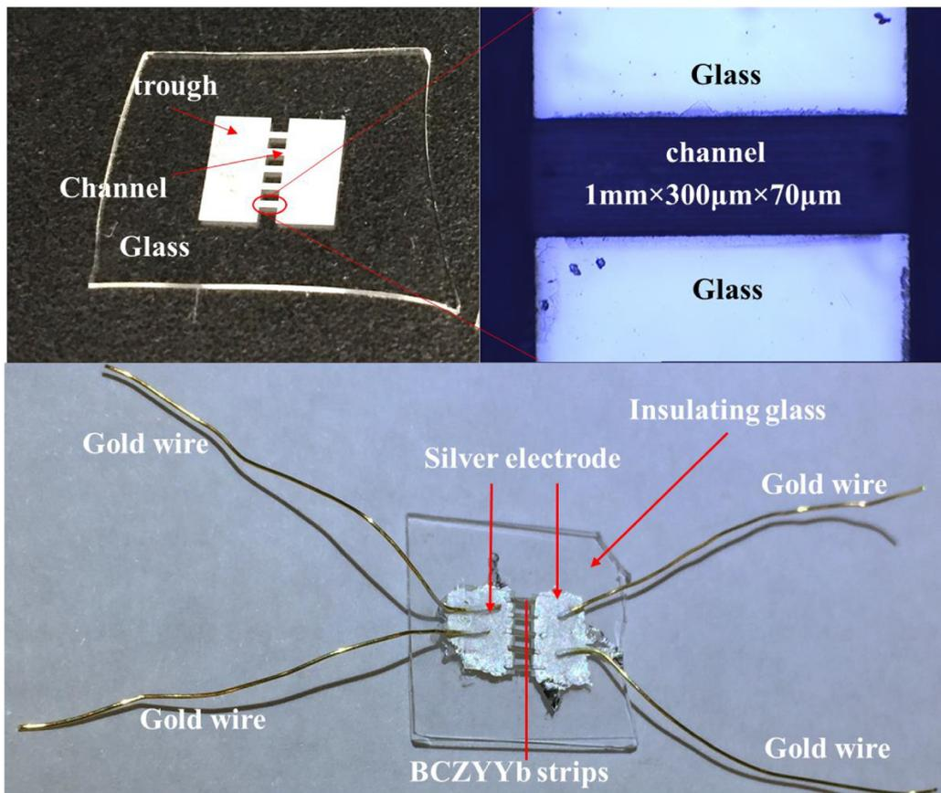
**Fig. 2.** Five BCZYYb strips after the removal of the porous edges were assembled into five glass channels. The two bigger troughs were designed to connect the channel ends for introducing silver electrodes. The design provided large cross section area and enough mechanical strength for measuring conductivity using electrochemical impedance spectroscopy under different conditions.
