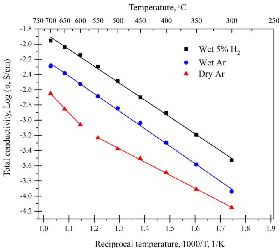
Fig. 10. Total in-plane conductivities of five-strip dense BCZYYb samples measured by EIS at 300–700 °C under wet 5% H<sub>2</sub> balanced by Ar, wet Ar, and dry Ar. The wet atmosphere was obtained by flowing through room temperature bubbler.
