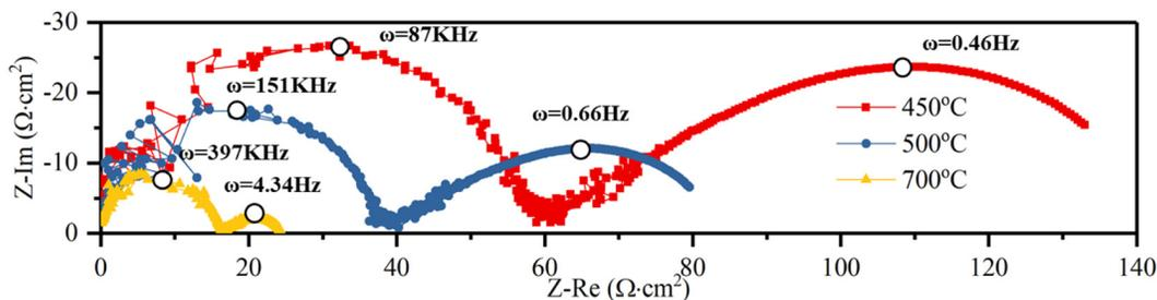
Fig. 9. Nyquist plot for electrochemical impedance spectroscopy for BCZYYb sample under wet 5% H<sub>2</sub> balanced by Ar at different temperatures.
