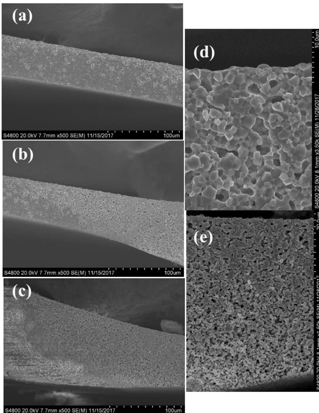
**Fig. 6.** Microstructures of BCZYYb strips with dense center and two porous edges. (a) dense center, (b) right porous edge, (c) left porous edge, (d) high magnification dense center, and (e) representative porous edge.
