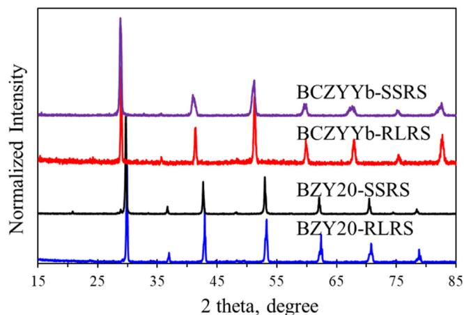
**Fig. 3.** XRD patterns of the protonic ceramic strips fabricated by rapid laser reactive sintering technology ( $< 10$  s), comparing with the protonic ceramic pellets fabricated by solid state reactive sintering (12 h at 1400–1500 °C). The XRD samples were fine powders ground from respective strips and pellets.
