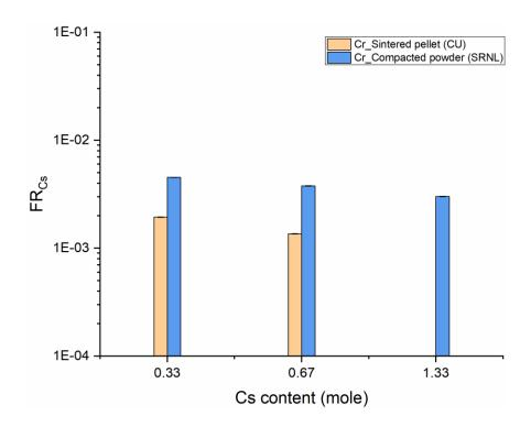
Figure 5. Fractional release (FR) of (a) Cs, (b) Ba, and (c) B-site substitutions for the Cr-, Ga, Fe-, Al-, and Zn-substituted hollandite samples. The ARM value is reported for comparison. The averaged FR values of the replicates are reported, and the error bars indicate the minimum and maximum measured values. Note: The Cs content is based on nominal stoichiometry. 11–15
