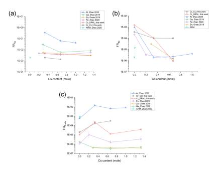
Figure 6. Various ratios of measured elemental release (a) Cs/B-site cation, (b) Ba/B-site cation, and (c) Cs/Ba after seven days of leaching. Note: the dashed bars indicate the stoichiometric ratios between different elements. 11–15
