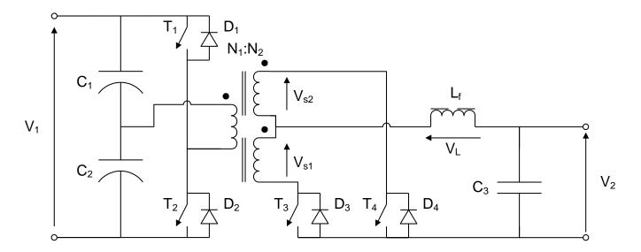
This converter configuration is very suitable when high voltage ratios are required (better sizing of the converter and high efficiency)
