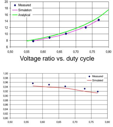
Efficiency vs. duty cycle
