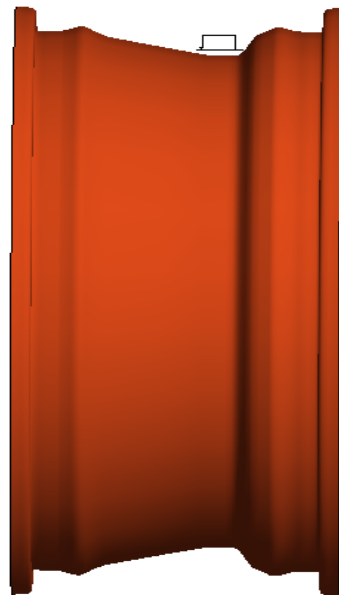
Fig. 2. Model for loop antenna above a metal rim
