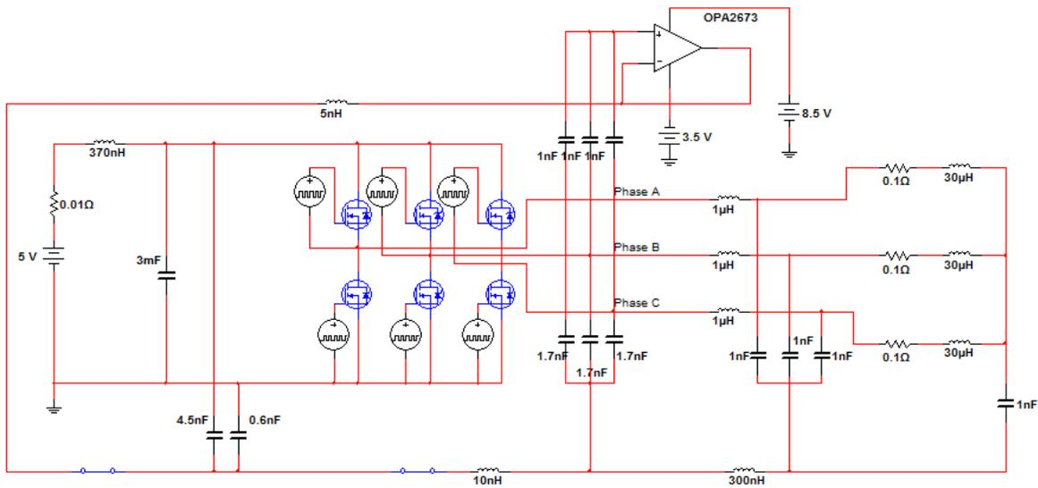
Fig. 2-31. Active balancing scheme.
