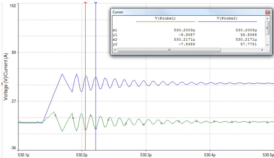
Fig. 2-27. Zoomed in simulation result w/o add-on capacitor.
