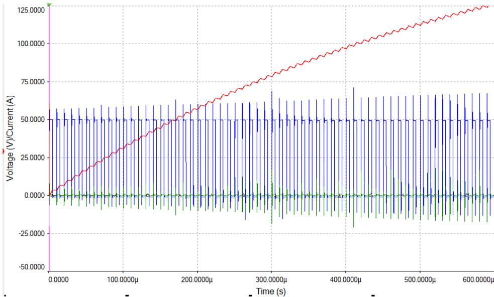
Fig. 2-26. Simulation result w/o add-on capacitor.
