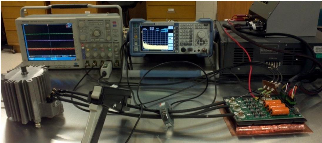
Fig. 3-2. CA6 inverter test setup.
