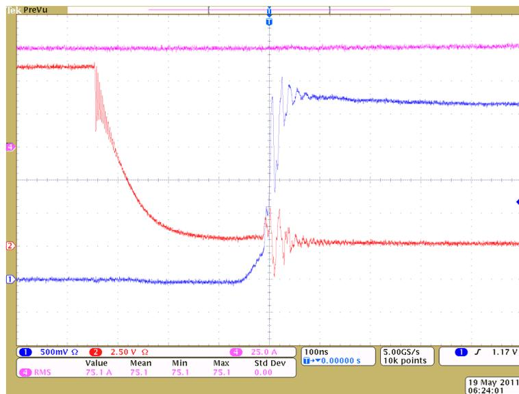
Fig. 22-18. Ringing on Phase A with 75-A current.
