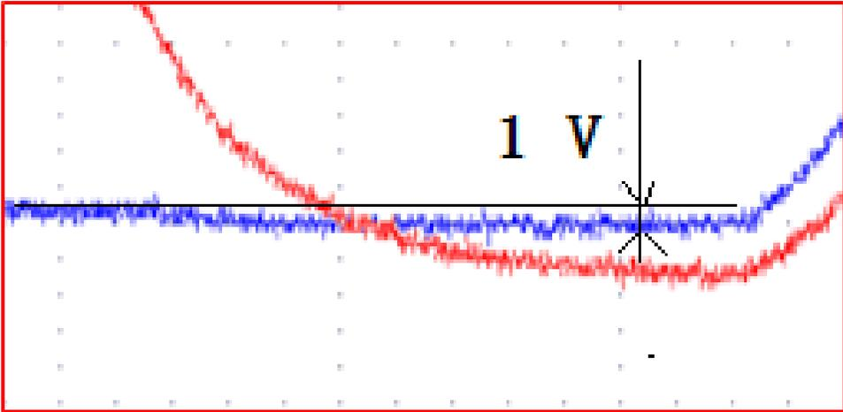
Fig. 2-6. Voltage while MOSFET body diode is conducting.
