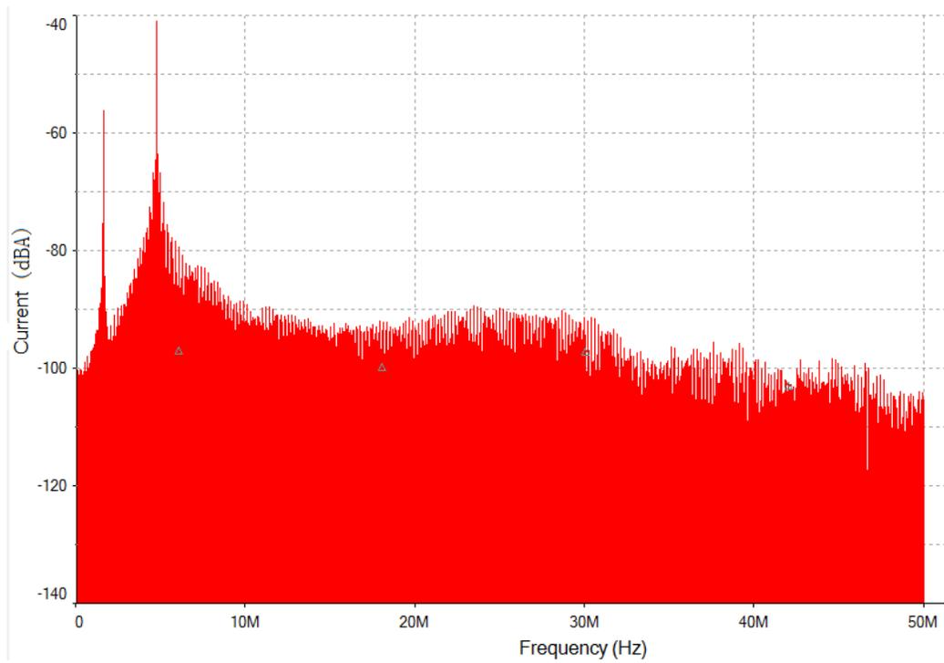
Fig. 2-34. Simulation of CM current w/ active balancing.
