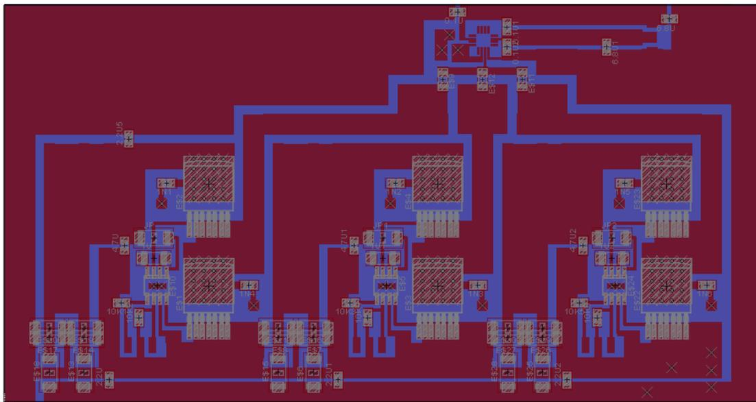
Fig. 2-32. Active balancing test board layout.
