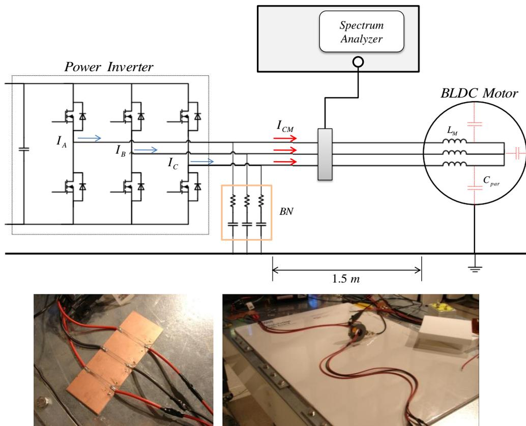
Fig. 3-1. Schematic representation of a passive balancing network (in gold box above) and photos of a prototype implementation used for preliminary evaluations.
