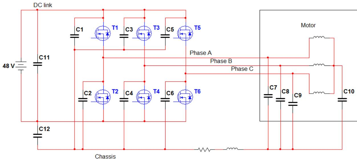
Fig. 2-8. Parasitic capacitance model.
