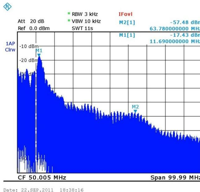
Fig. 2-29. Measure common mode current showing broad hump at 60 MHz.
