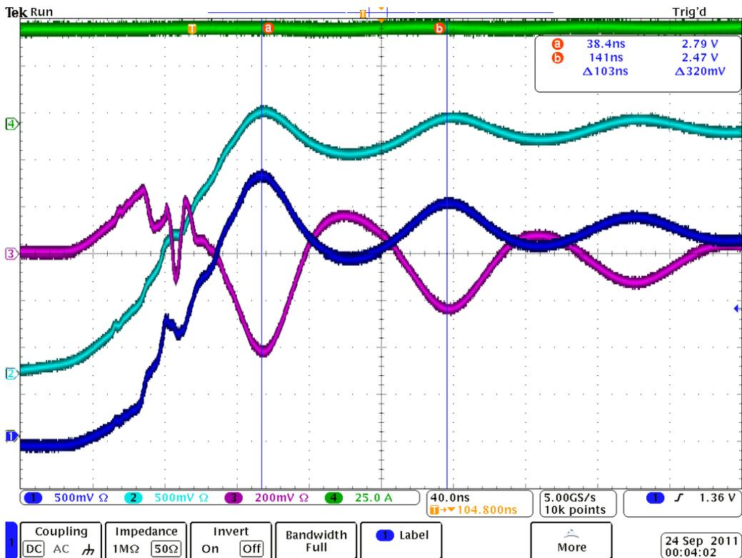
Fig. 3-23. Ringing frequency shifted on Phase A with SMD 0.1uF capacitor.
