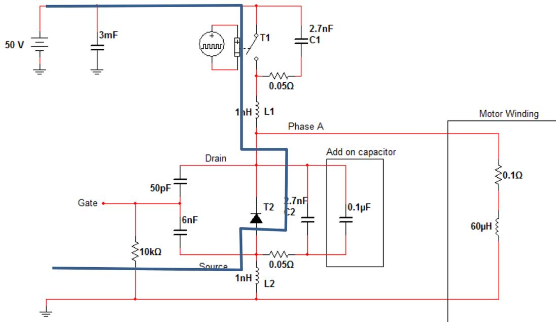
Fig. 2-25. SPICE simulation of ringing on Phase A.
