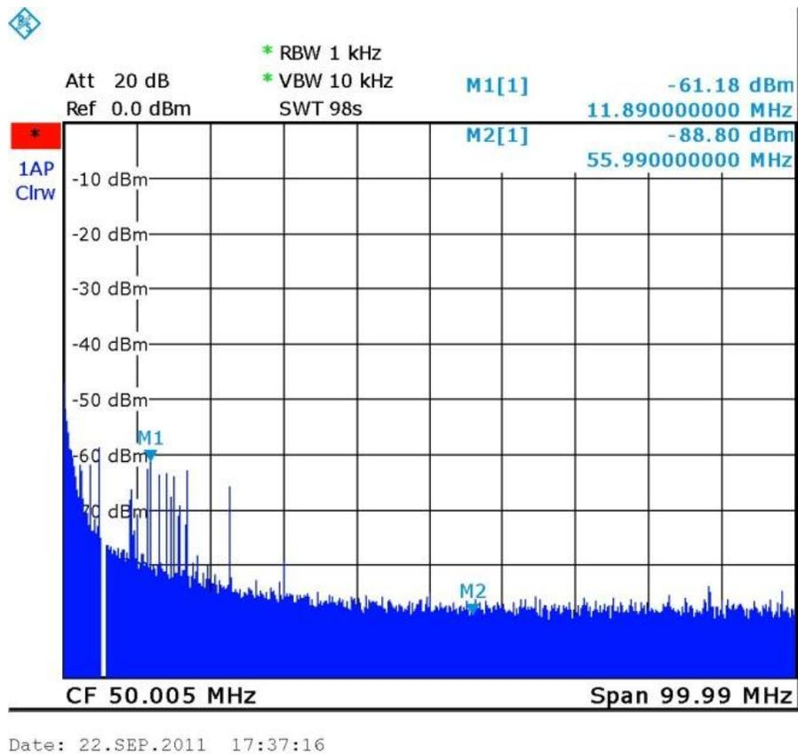
Fig. 3-3. Common-mode current measurement noise floor.
