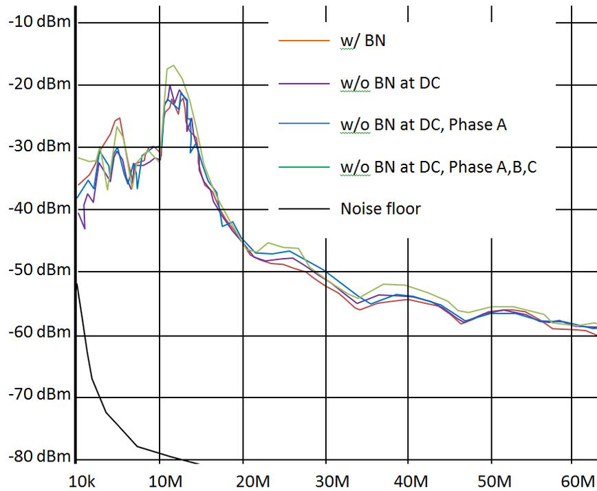
Fig. 3-9. Measured CM current with inverter in the CBA 110 state.
