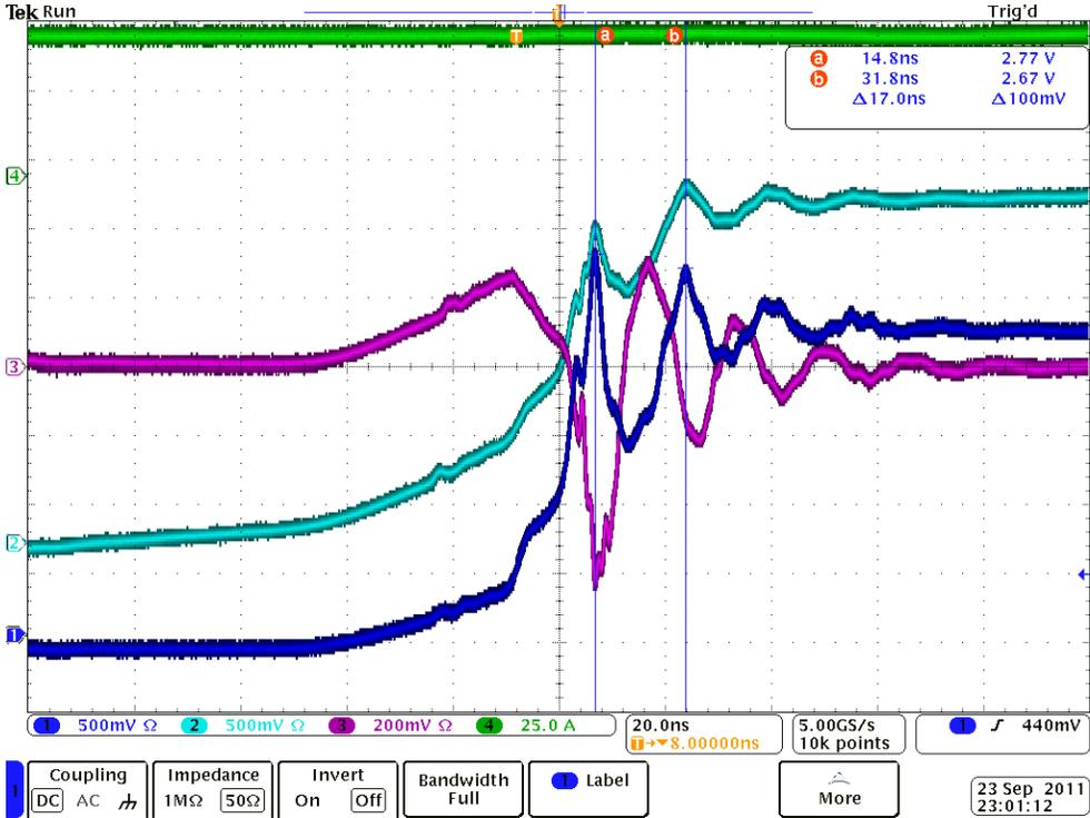
Fig. 2-21. Ringing frequency without add-on capacitor.
