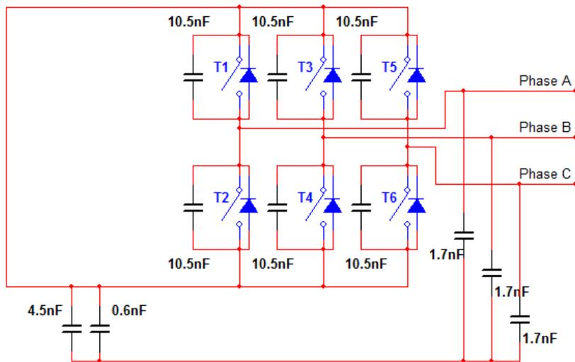
Fig. 2-11. CA6 Parasitic capacitance estimation.
