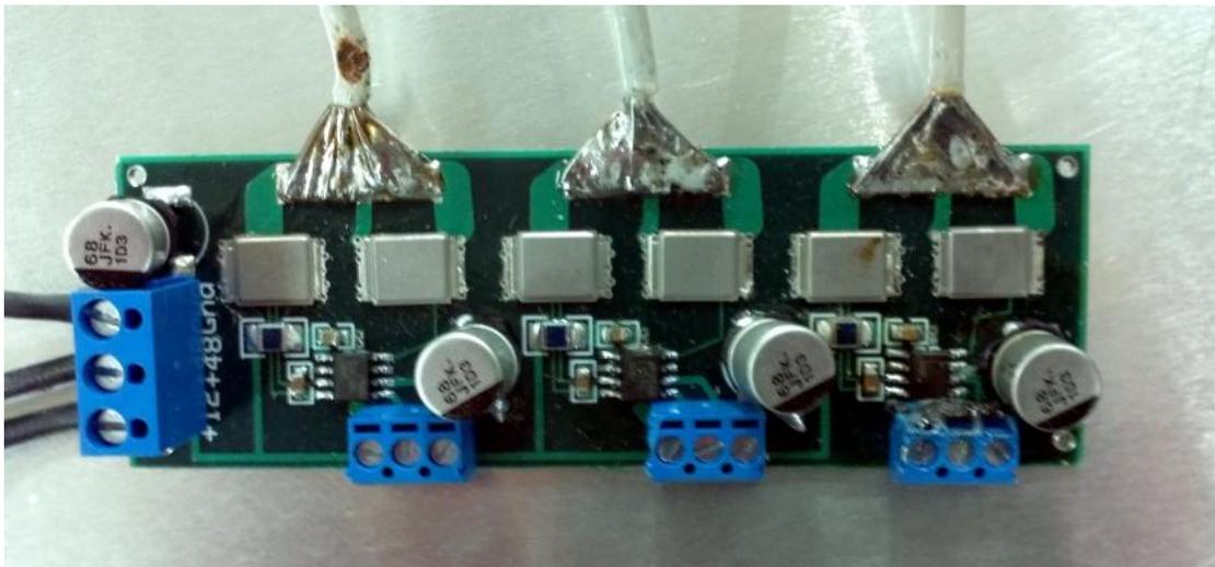
Fig. 4-30. Prototype board used to evaluate alternative MOSFET configurations.
