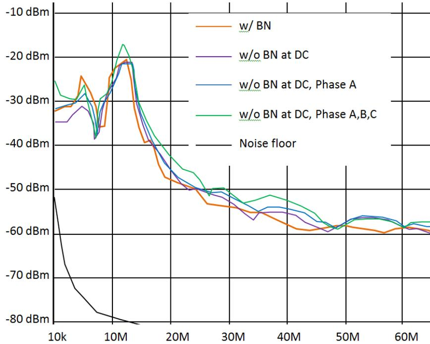
Fig. 3-8. Measured CM current with inverter in the CBA 001 state.
