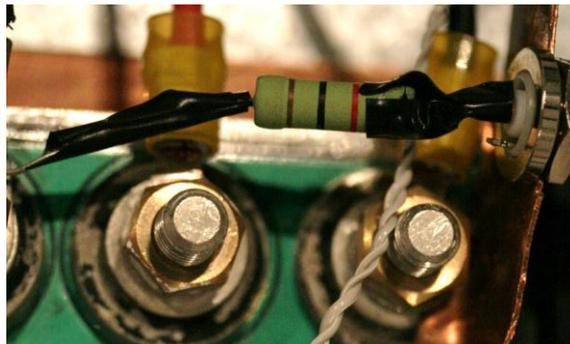
Fig. 2-12. Customized voltage probe.
