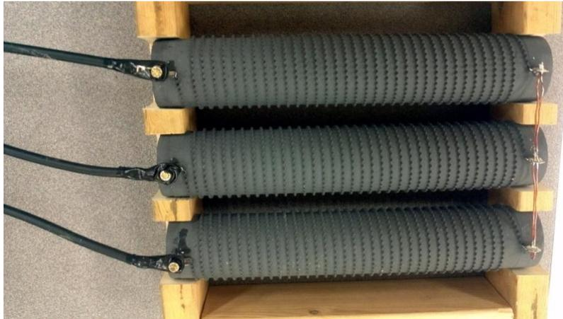
Fig. 2-19. Resistive load used to replace the motor.
