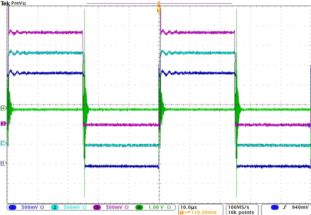
Fig. 2-13. Common mode current in time domain.
