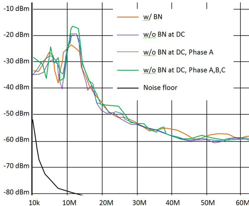
Fig. 3-10. Measured CM current with inverter in the CBA 011 state.
