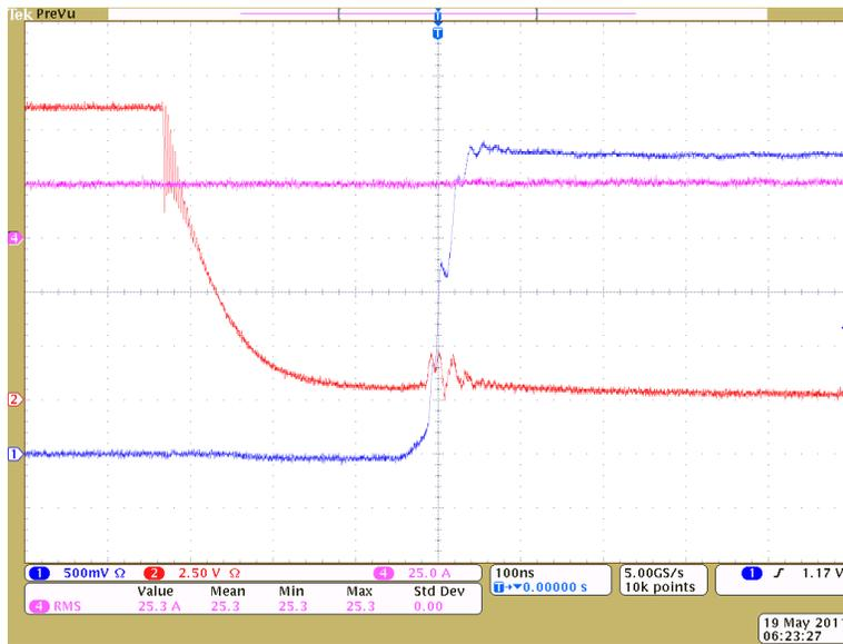
Fig. 2-17. Ringing on Phase A with 25-A current.
