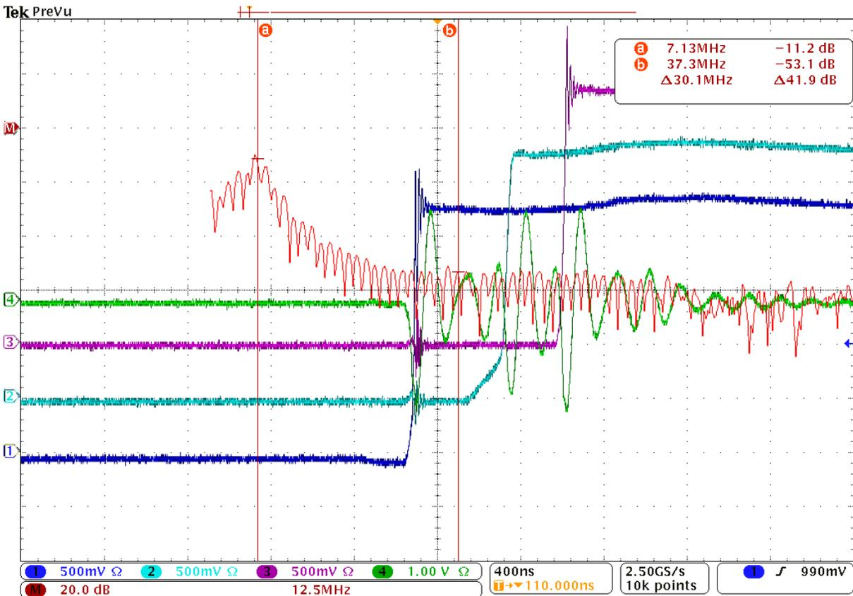
Fig. 2-16. Common mode current in time domain with extended phase wires.
