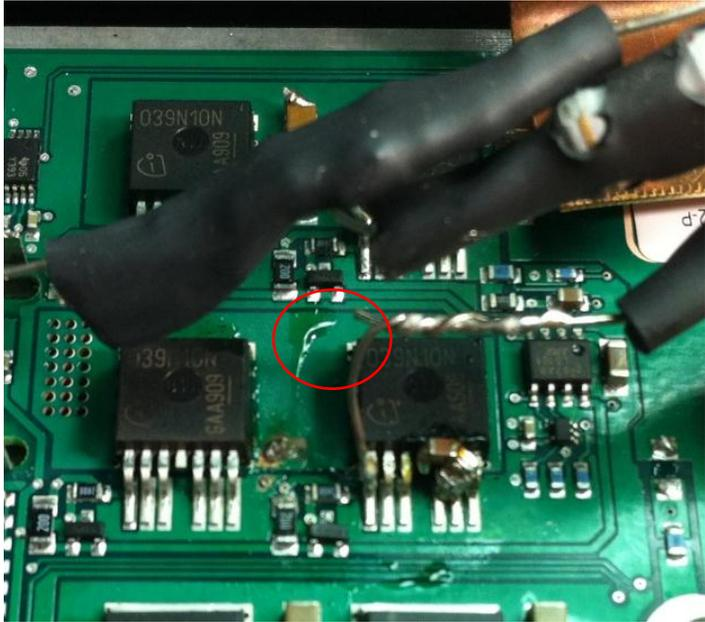
Fig. 2-20. SMD Capacitor added to MOSFET.
