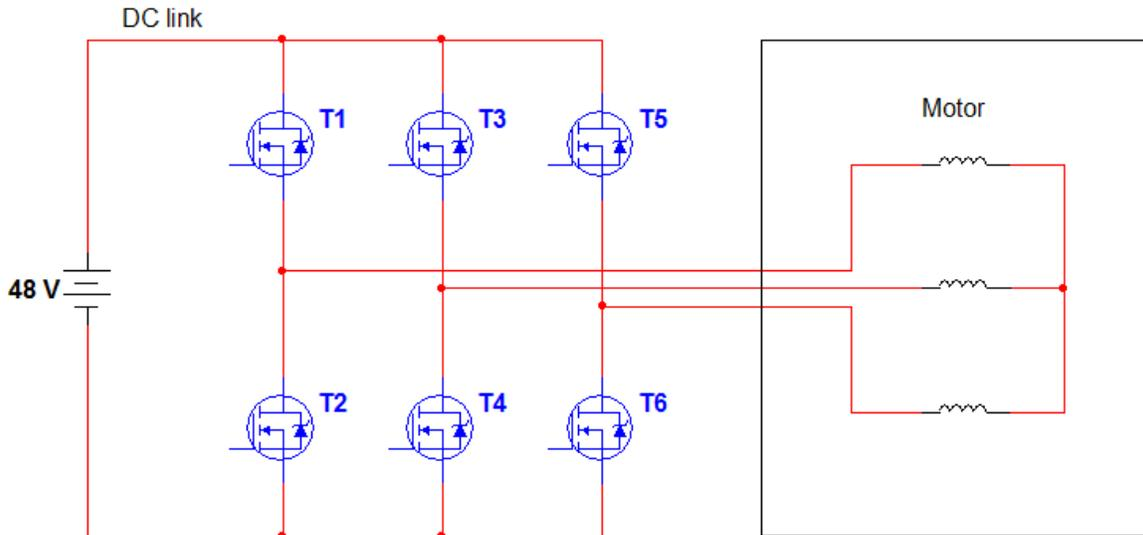
Fig. 2-3. MOSFET motor interface.
