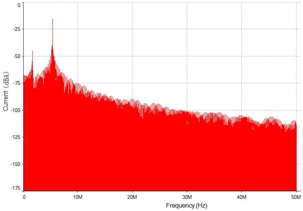
Fig. 2-33. Simulation of CM current w/o active balancing.
