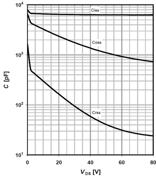
Fig. 2-24. Typical capacitances of IPB039N10N3 (From datasheet).
