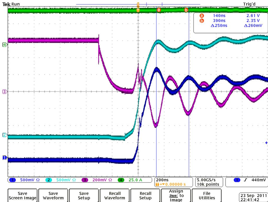
Fig. 2-22. Ringing frequency shifted on Phase A with SMD 1uF capacitor.
