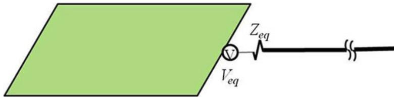
Fig. 6 I/O coupling model with CM source and impedance
