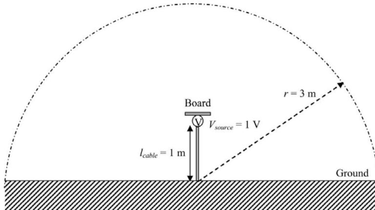
Fig. 7 Board-source-cable geometry
