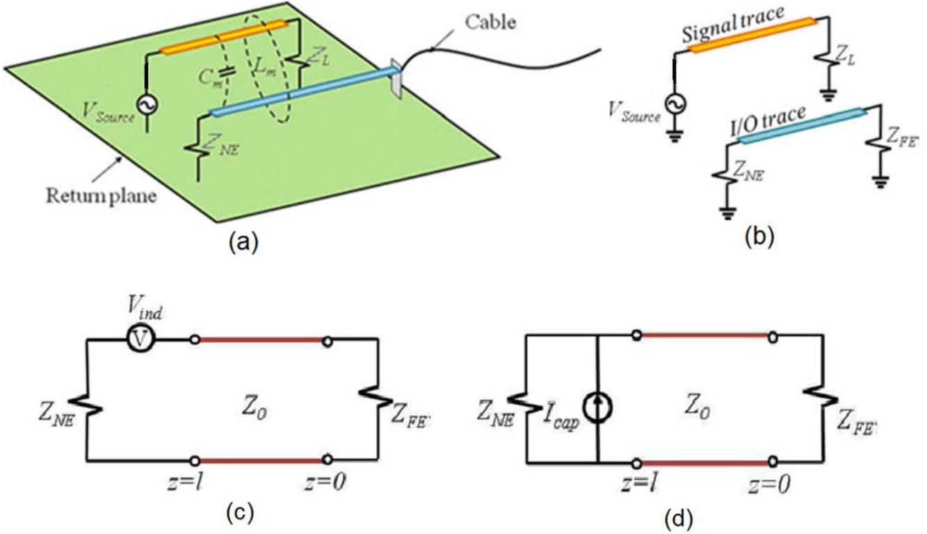
Fig. 3 Coupling algorithm: (a), coupling model, (b), simplified model, (c), inductive coupling schematic, (d), capacitive coupling schematic.
