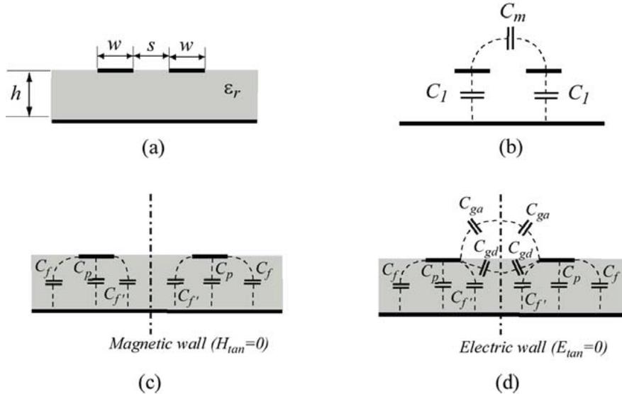
Fig. 4 Configuration of coupled microstrip line (a), general equivalent circuit (b), and breakup of even mode (c) and odd mode (d) capacitance
