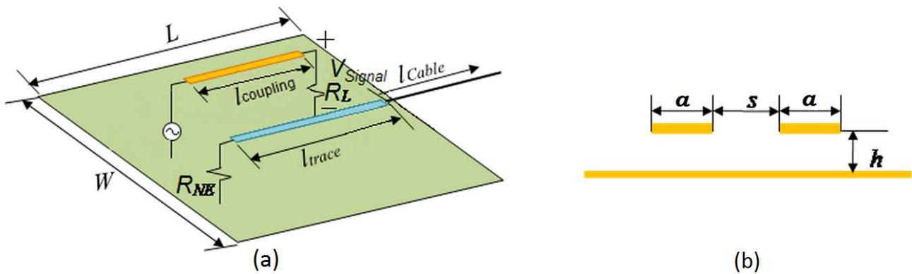
Fig. 1. I/O Coupling model: (a), top view, (b), section view.
