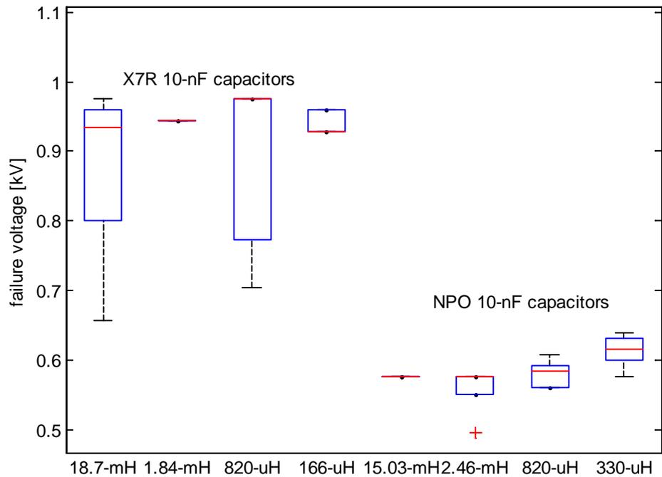
Fig. 6. Failure voltage of 10-nF capacitors grouped by value of the test inductor.
