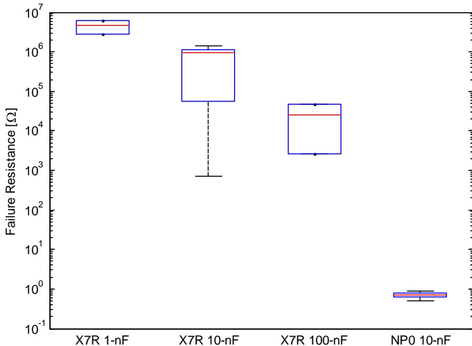
Fig. 8. Insulation resistance measured after the failure pulse.
