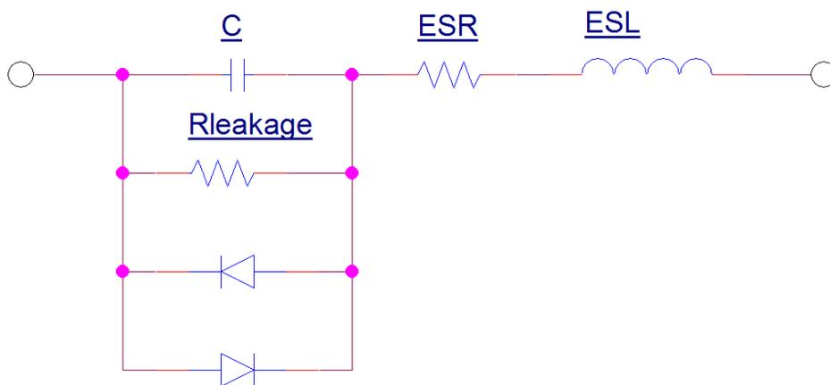
Fig. 15. Equivalent circuit of a failed X7R capacitor.
