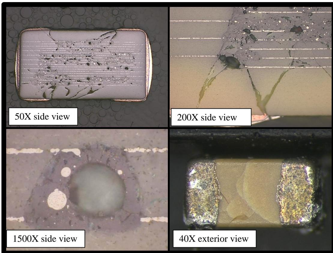
Fig. 13. Damage to an X7R capacitor exposed to 5000 pulses after the initial failure.
