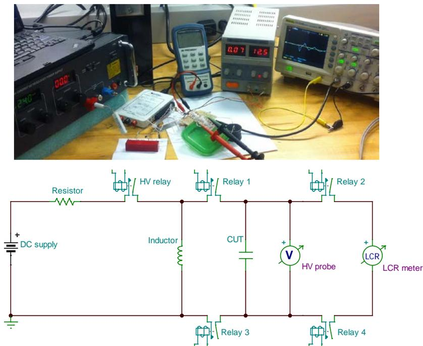
Fig. 1. EFT test configuration for MLC capacitors.
