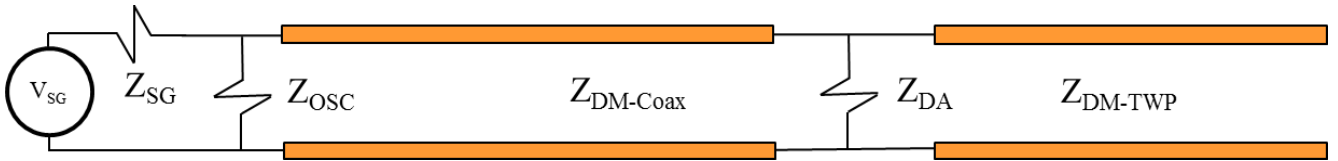
Fig. 7. Equivalent circuit for measurement set up.
