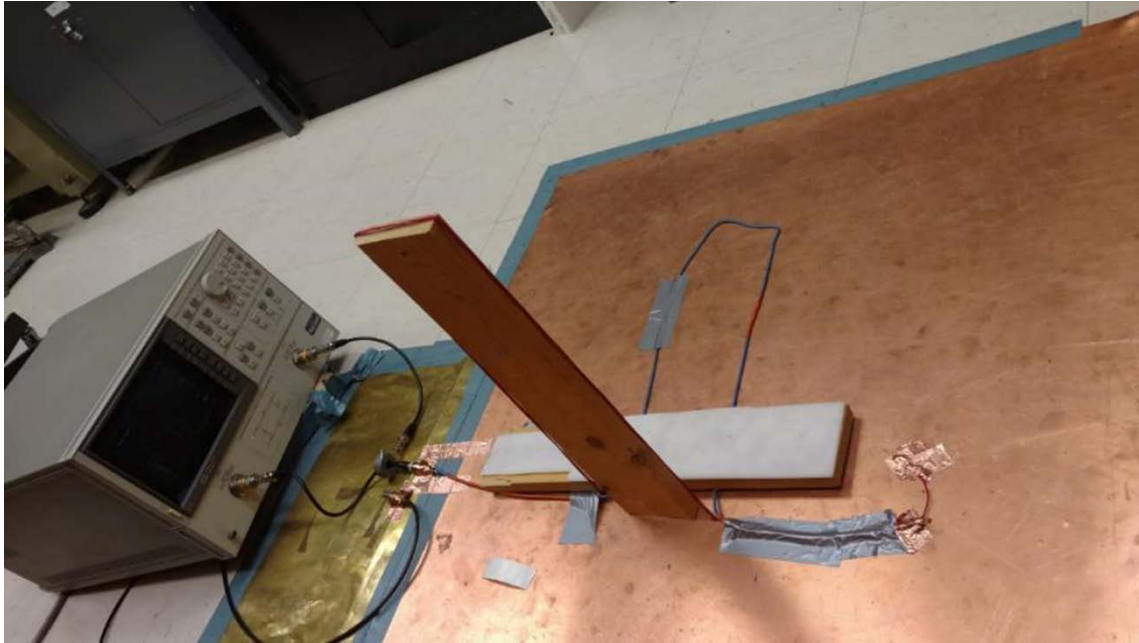
Fig. 9. Test set-up for the detached twin wire pair from the ground wire.
