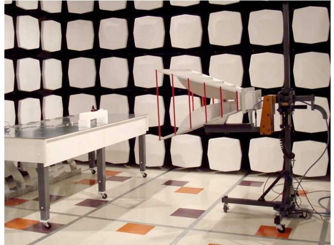
Fig. 1. CISPR 25 radiated emissions test configuration.
