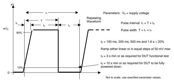
Figure 3: Supply Voltage Ramp Up Test
