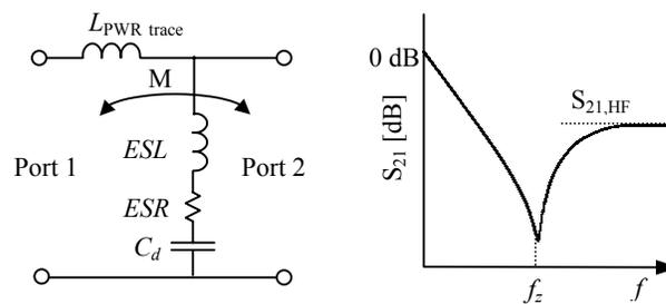
**Figure 1. Equivalent circuit for a decoupling circuit and its transfer coefficient,  $S_{21}$**
