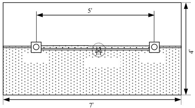
(b) Test board with one return path
