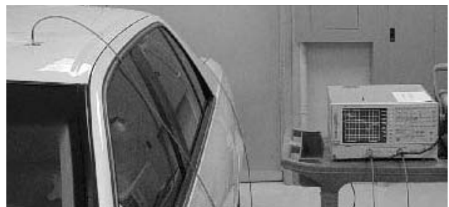
Fig. 1. Experimental setup. Cavity resonances were measured with a network analyzer using antennas placed into the passenger compartment.
