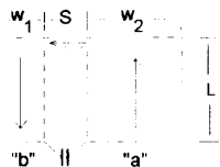
Figure 11: Capacitor added across return plane gap at input of coplanar strip transmission line
