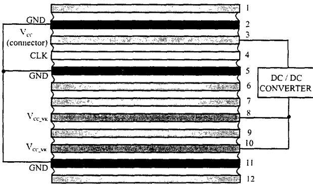
Figure 3. Layer stack-up for the CPU #2 PCB module.
