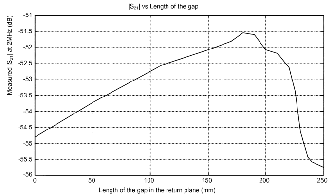
Fig. 8. |S_{21}| for inductive crosstalk as a function of the length of the gap in the return plane. The test board was 250 mm long and the length of the coupled traces was 190 mm.
