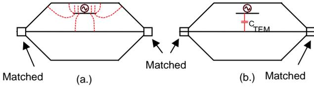
Fig. 2. Electric field coupling between an IC and a TEM cell.
