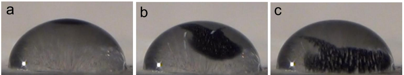
Figure S5. Dynamics of cluster settling in the droplet with 100 nm beads of 0.2wt% after the field removal. The time interval between frames is 6 seconds.
