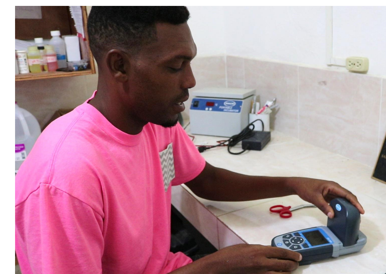
Figure 6. Levels of free chlorine are tested in a water testing laboratory using the HACH DR 900 Colorimeter.
