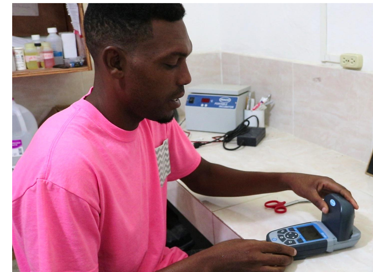
Figure 6. Levels of free chlorine are tested in a water testing laboratory using the HACH DR 900 Colorimeter.
