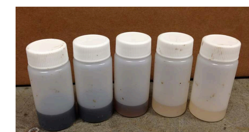
Fig. 8: Left to right: Unfiltered CNS and CNS after filtration through 0.8, 0.22, 0.1, and 0.05 µm MCE membranes.
