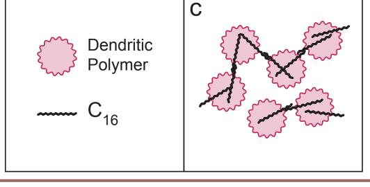
Proposed schemes of C16 complexation with dendritic polymers. (a) C16 molecules are partitioned into dendritic polymers. Potential interactions leading to super-complexes include (b) C16 capping by dendritic polymers and (c) C16 end-to-end complexation, both through hydrophobic interactions
