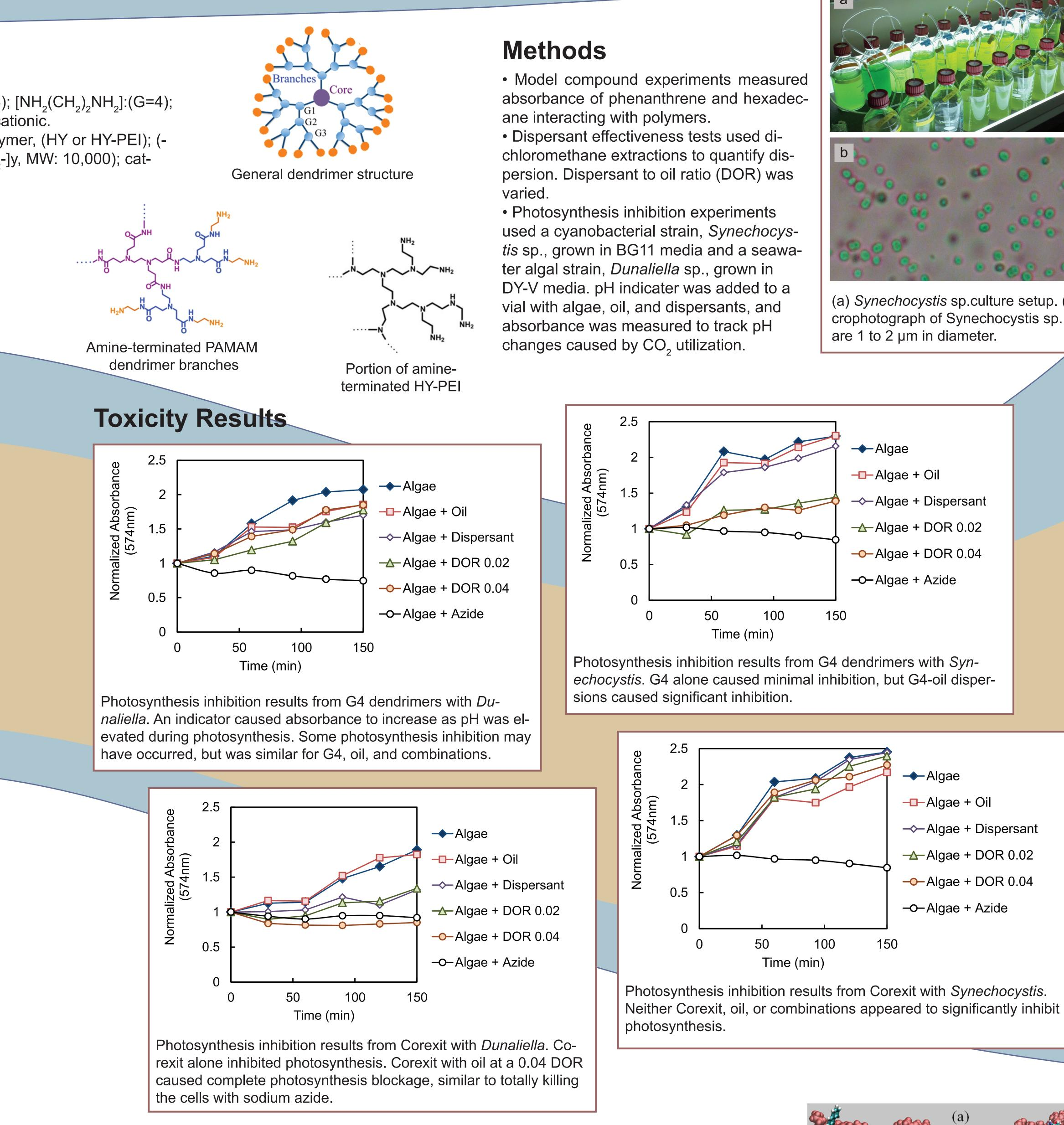
Dendritic polymers demonstrate oil-dispersing effectiveness due to their hosting capacity for hydrocarbons. The amphiphilic nature of the polymers allows them to remain soluble even after hydrocarbon capture.
