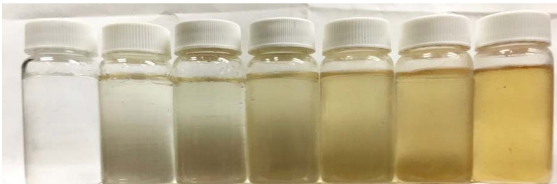
Figure 3-10. The vials containing the blank followed by the six solutions used for Corexit's calibration curve.
