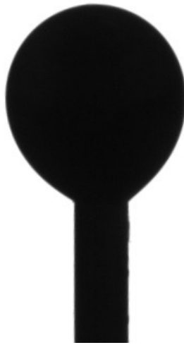
Figure 3-8. A screenshot of the live video of the oil droplet that is analyzed by DSA to determine the IFT between the oil droplet and water.
