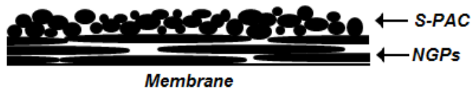
Figure 5.33. A representation of a layer-by-layer assembly of adsorbents. Figure not drawn to scale, and although the manufacturer of the NGPs describes them as platelets, they may in actuality adopt more spherical shapes as a result of aggregation.
