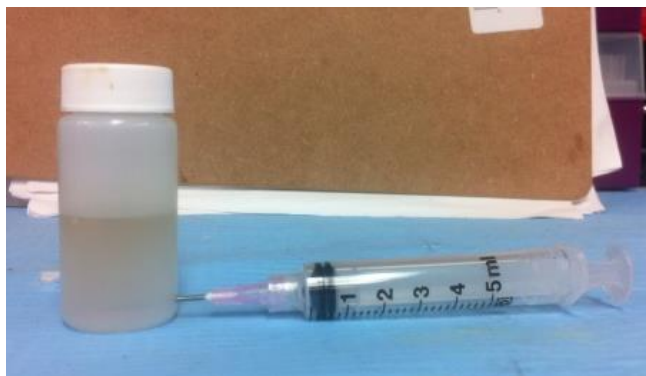
Figure 4-1. In some experiments, 3 ml water sub-samples with dispersed oil were extracted from the bottom of plastic vials using a needle penetrate through the vial.
