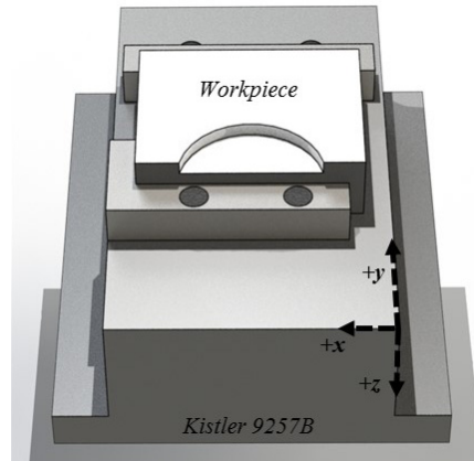
Fig. 5. Milling test setup for experimental validation.
