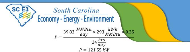
The *electricity consumption savings* (ECS) per year with the plant's operation of 8760 hours per year is
