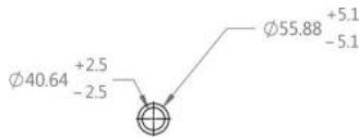
Figure 5 The maximum diameter of an object the robot can pass is 55.88 mm
