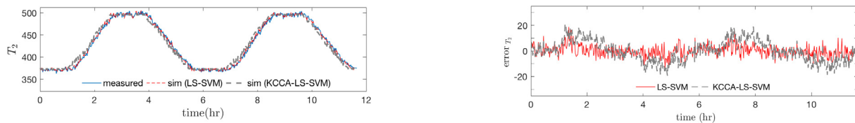
Fig. 5. Example 2: (left) Validation results for CSTR output temperature T_2 (°C) using LS-SVM-based identification with and without full states measurements, and (right) validation error.
