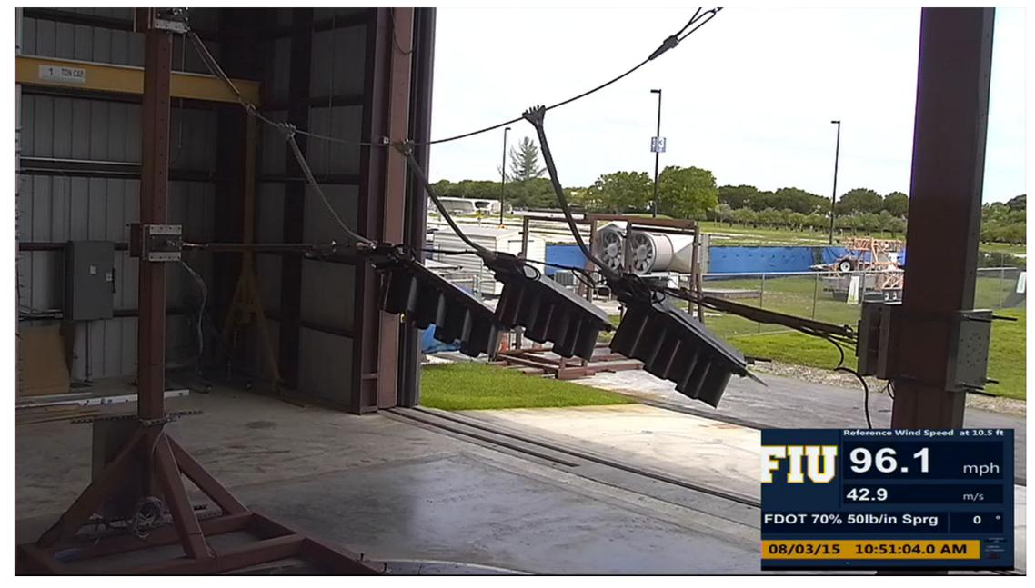
Findings: Instability sets in at critical wind speed causing failure.
