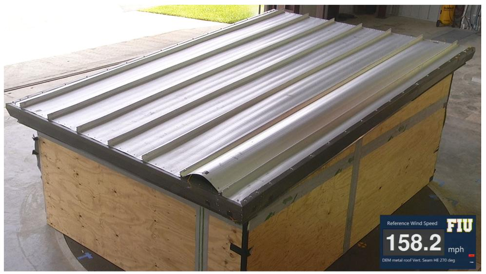
**Findings:** Considerably higher suctions with larger non-uniformity for trapezoidal roof; The panel vibrations in the trapezoidal roofs crept into the panel-ribs causing high deflection and failure.
