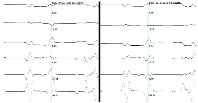
Fig. 5: Comparison of raw sensor data during a bite of the finger mounted sensor (left) and the wrist mounted sensor (right).
