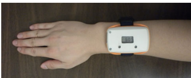
Fig. 4 Prototype device using MEMS gyroscope
