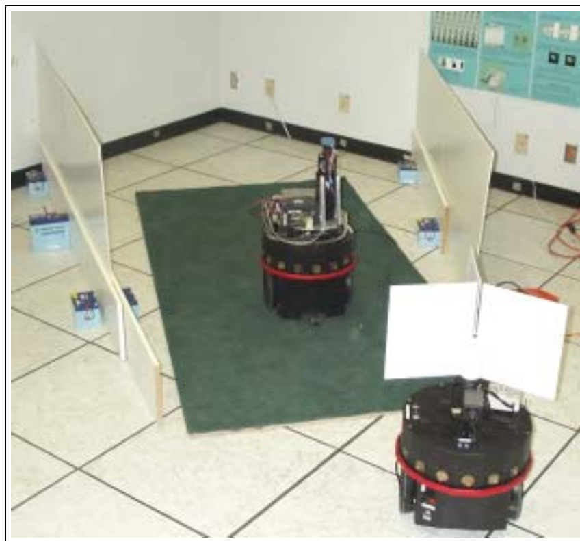
Figure 9: Measuring the odometry error on carpet.
