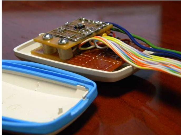
Figure 2.15 Sensor comprised of two gyroscopes and one accelerometer.
