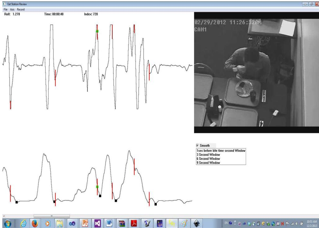
Figure 2.5: The developed software for bite detection
