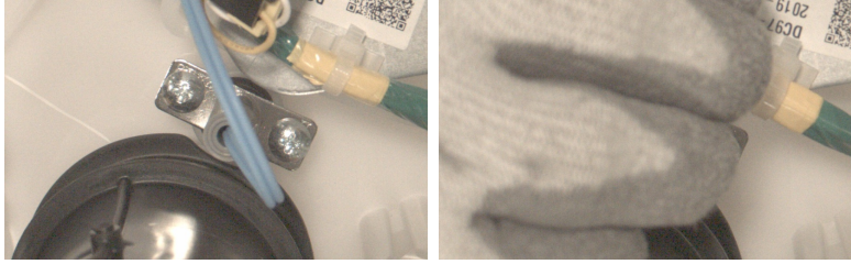
Figure 2.10: In the first figure, the thermistor frame is screwed into the tub completely (OK). In the second figure, there is a human hand covering the part and we cannot inspect it (NOK).
