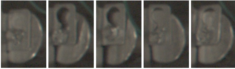
Figure 1.5: Variability in appearance due to incorrect assembling.
