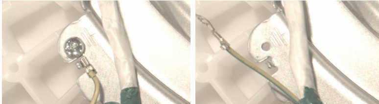
Figure 2.11: In the first figure, the screw is screwed tightly on to the frame (OK). In the second figure, the screw is absent (NOK).
