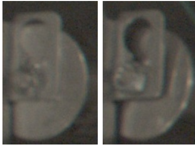
Figure 3.13: An OK and an NOK image of the EMI filter.
