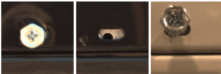
Figure 2.13: Screws on the back of the washing machine. The first figure is an OK screw. Next, the screw is absent (NOK). In the last figure, the screw is not screwed into the frame (NOK).
