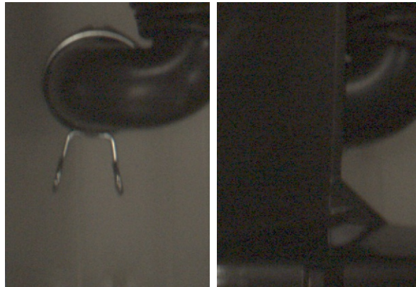
Figure 2.5: In the first figure, the hose is seated on the tub and the clamp is secure (OK). Next, it is occluded by an object and it cannot be inspected (NOK).
