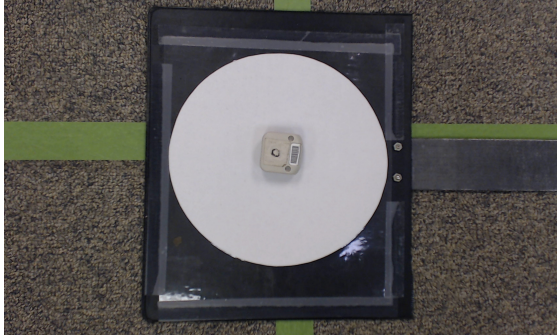
(a) White target circle with Ubisense tag
