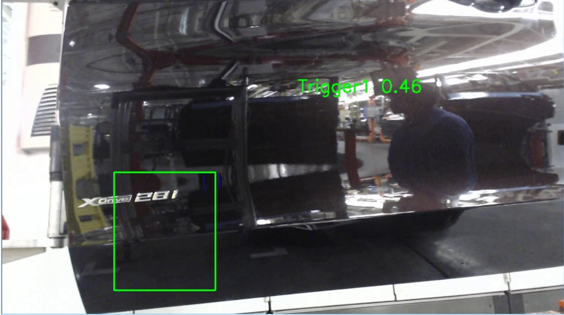
Figure 3.31: A screen grab of the setup program running the post-bump video with the original templates on the door line. The template does not appear within the trigger search window.
