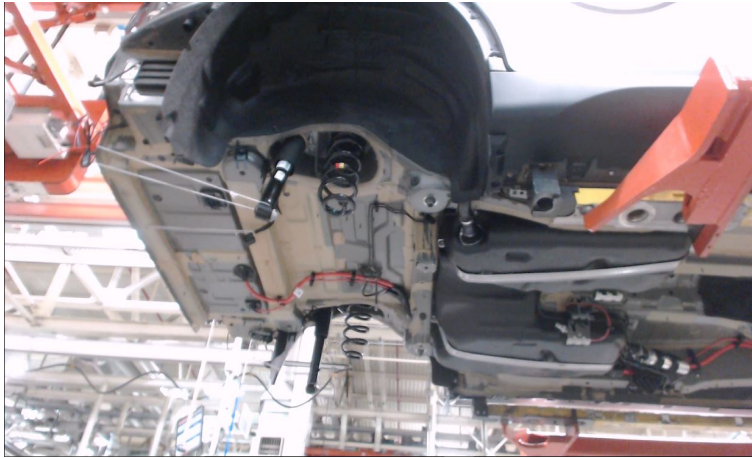
(a) Spring coil correctly installed.
