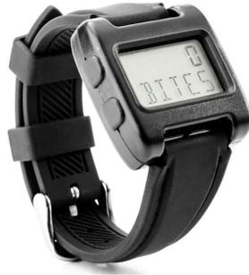
Figure 1.1: The ELMM watch, one example of a wearable wrist based device that can track energy intake through bites.
