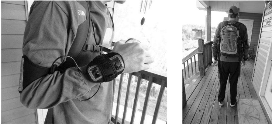
Figure 1.11: Wrist activity tracker connected to a laptop carried in a backpack [55].
