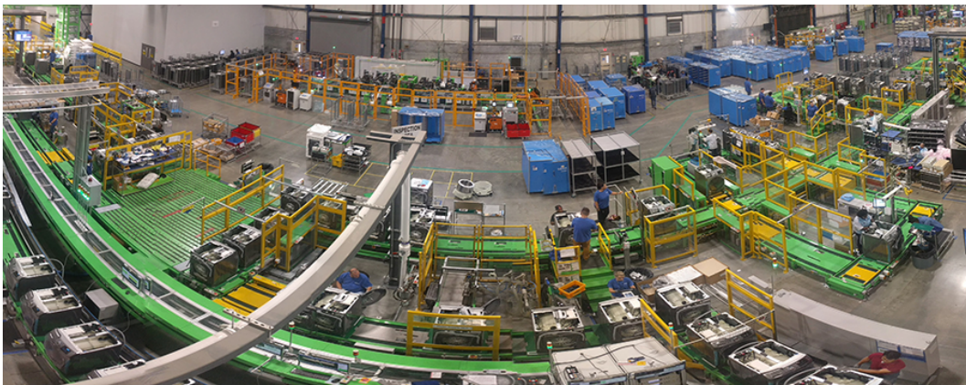
Figure 2.2: Overhead panoramic view of front-load washing machine assembly line at SEHA plant.
