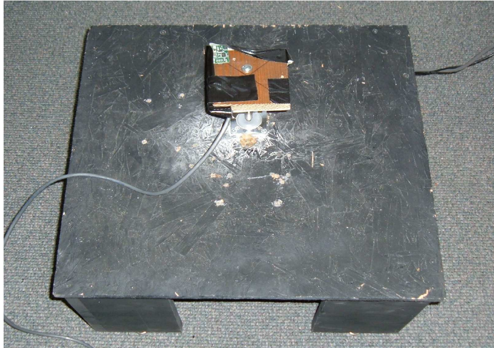
Figure 2.1: The turntable apparatus built with a sensor attached.
