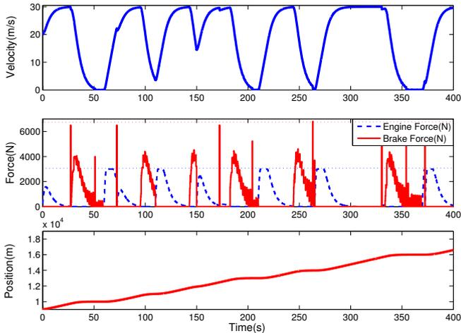
Fig. 5. Velocity, Control Inputs and the Position for a vehicle without advanced signal information.
