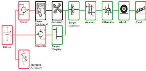
Fig. 3. Schematic of a PSAT powertrain model
