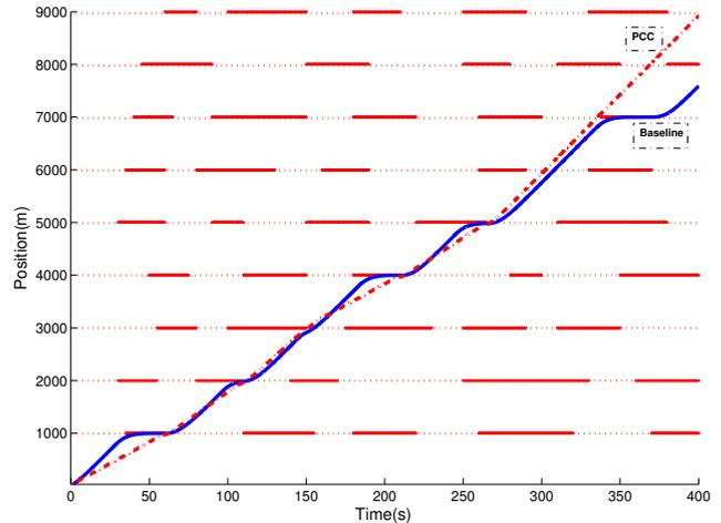
Fig. 4. Trajectory of PCC and baseline vehicles with respect to the red-light map.
