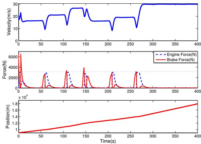
Fig. 6. Velocity, Control Inputs and the Position for a vehicle with advanced signal information.
