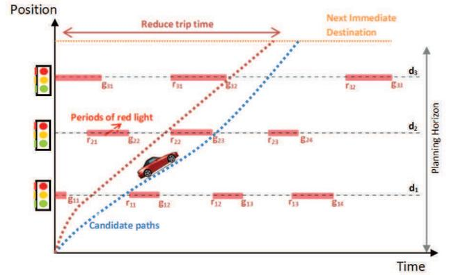
Fig. 2. Schematics map of red lights distributed over space-time. The graphics shows how a PCC car passes two consecutive intersection without having to stop at a red.
