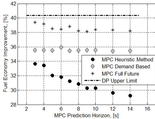
Fig. 5. MPC Horizon Variation - Comparison of Decay Methods
