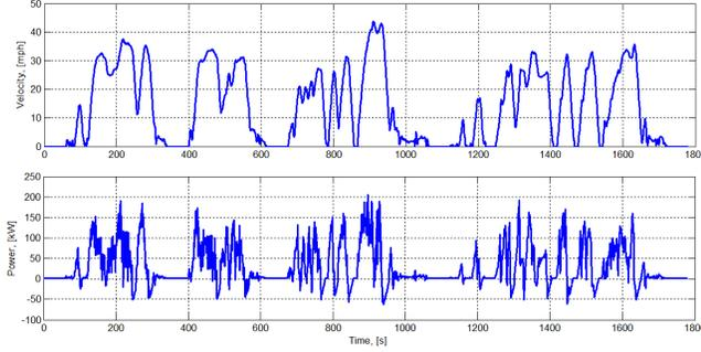
Fig. 1. Velocity and Power Profile for CSHVR Cycle
