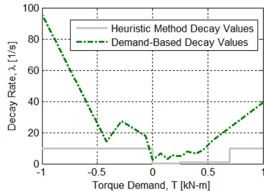
Fig. 4. Decay Rate Comparison, Heuristic vs. Demand-based Values
