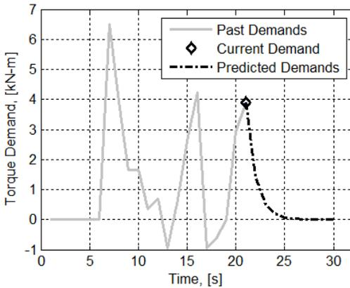
Fig. 2. MPC Prediction Method - Exponential Torque Decay
